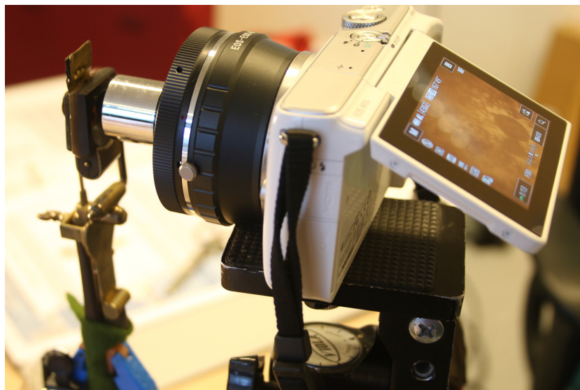
Figure 4. Set-up for photography with a Canon EOS M10 fitted with an eyepiece adaptor and fossil diatoms on the camera's screen.
