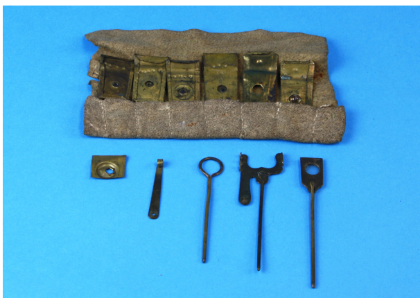
Figure 3. The lenses, lens holders and sample holders belonging to the Van Musschenbroek microscope used in this study. The dots engraved on the sample holders indicate the strength of the lens.
